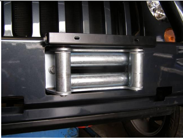
Roller Fairlead installed
